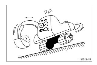
Avoid parking and stopping on a slope. Lower the grapple to the ground and block the track when parking.
