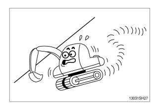
The engine angularity limits are 35 degree. Do not operate by more than the engine limits in any case.
